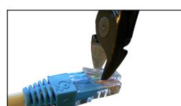
Cut off the prolongations of the lock-release on the RJ45 connectors to secure unauthorized disconnection of the CO2 Safety System.
