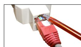
Use a small screwdriver to disconnect the RJ45 plugs.
