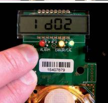
2. Press the lower button again until the current address is shown.
